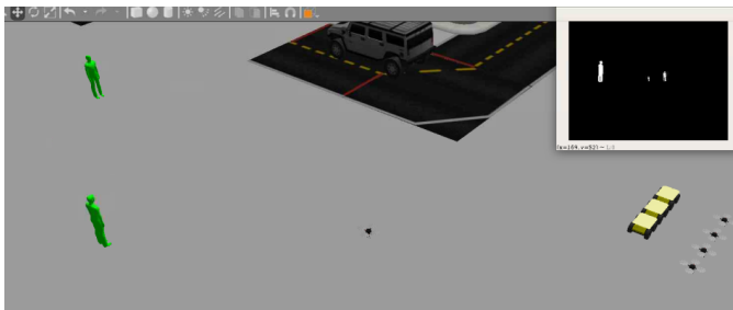
Fig. 3. Our moving drone -in black at the center of the simulation environment- is capturing the position of its targets, the green men. In the upper right corner is the mask obtained with the drone camera, on which we apply DBSCAN clustering to find all the targets
